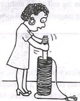
Fig. 4.50, It is more difficult to push the magnet into a coil with many loops because the magnetic field of each current loop resists the motion of the magnet.
